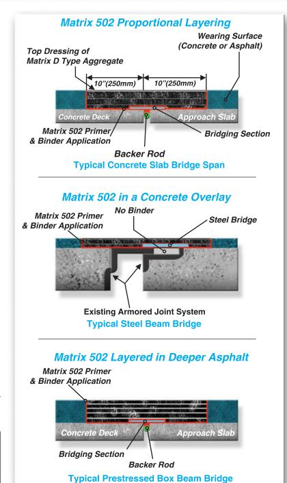
The Matrix 502 Asphaltic Plug Bridge Joint System meets requirements of ASTM D6297, Standard Specification for Asphaltic Plug Joints for Bridges.
